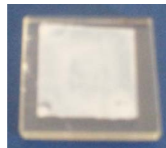
Fig 6: Image of the glass coated with TiO 2
